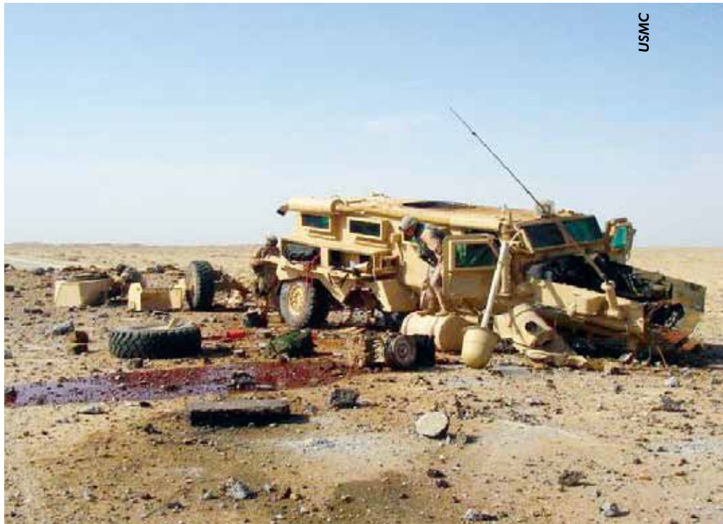
The MRAP focused on assuring the safety and survival of the vehicle occupants. This Marine Corps Cougar hit an IED suffering extreme damage yet all the occupants were uninjured.
