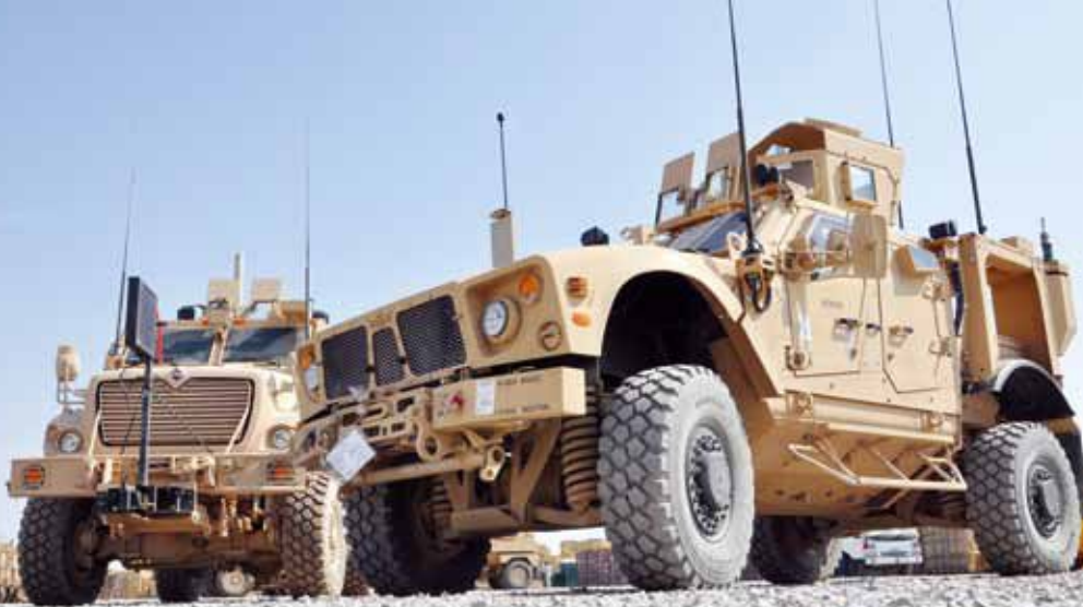
A new M-ATV mine-resistant, ambush-protected all-terrain vehicle, built specifically for the mountainous Afghan terrain, parks next to a larger MRAP, MaxxPro Dash in 2009.
