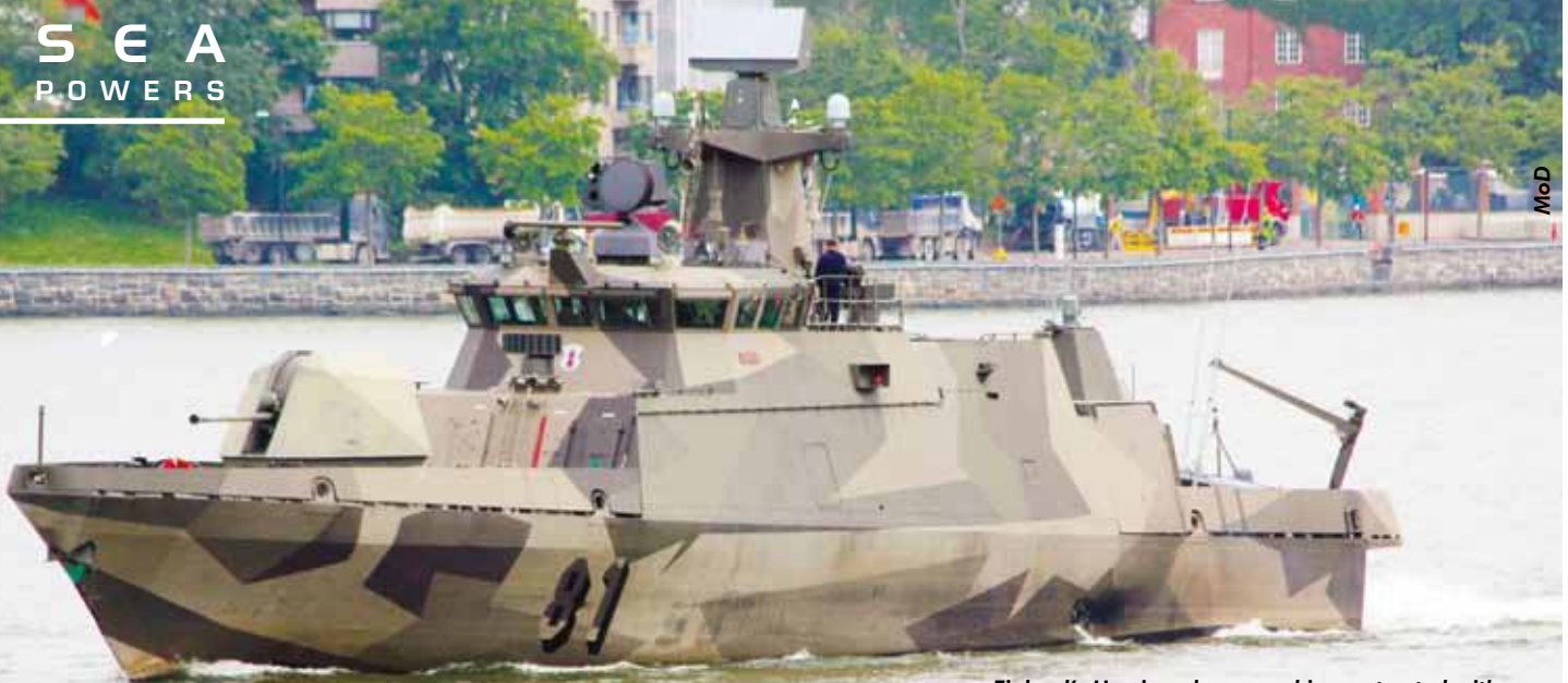
Finland's Hamina-class vessel is constructed with an aluminum hull and re-enforced carbon fibre composite superstructure. It is armed with a Bofors 57 mm/70 SAK Mk3, four Saab RBS-15 Mk2 SSMs and Denel Umkhonto-IR SAM.
